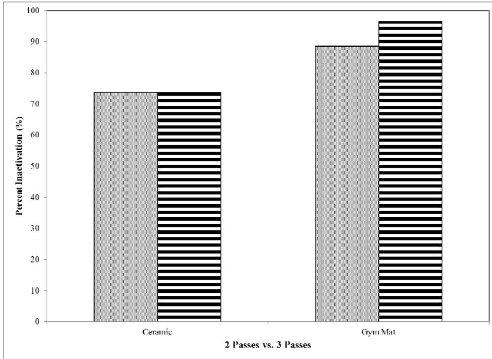
**Figure 3. Comparisons of Number of Passes at Half-Speed**
